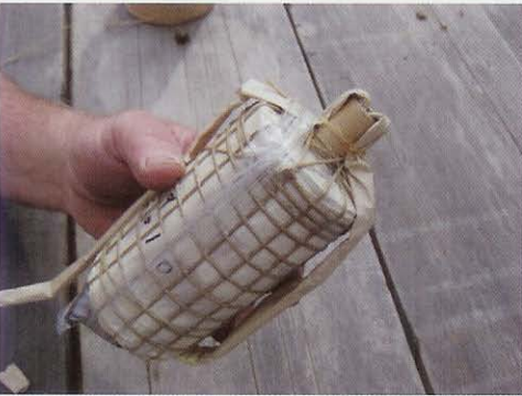
Photograph 34 – Securing the leader-passfire to the shell.
