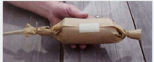
Photograph 36 – The wrapped shell before trimming the excess paper and application of the label.
