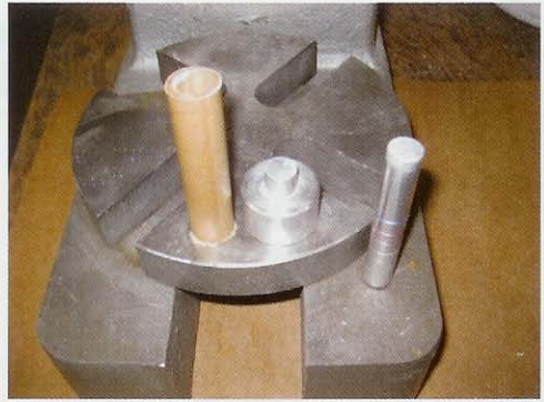
Photograph 4 – Note the ramming base with a riser to leave a 0.25 inch recess in one end.
