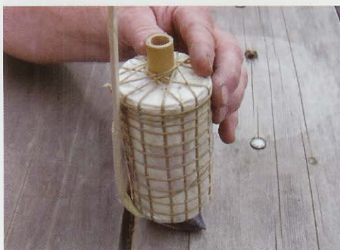
Photograph 31 – Estimating where the leader needs to be bared to light the whistle.
