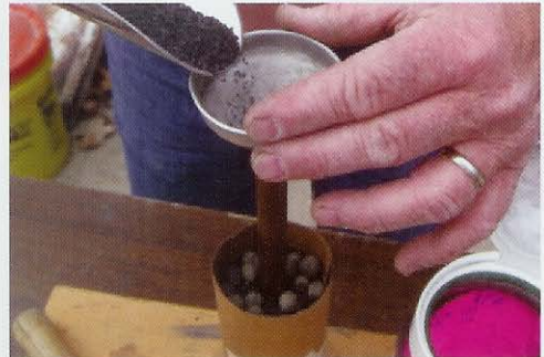
Photograph 16 – Adding the 4FA burst charge to the canulle.
