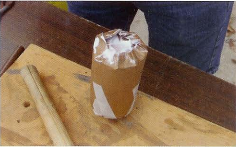
Photograph 19 – Overhanging paper pleated down.
