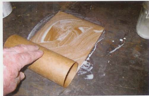
Photograph 2 – Rolling the case.
