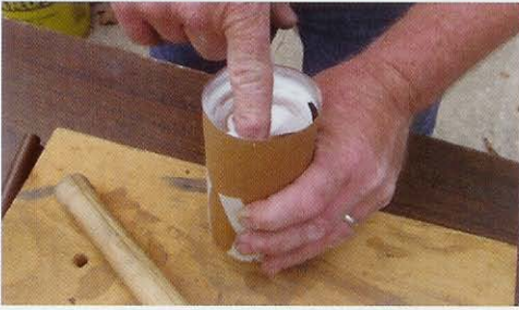
Photograph 18 – Gluing-in the end disk.
