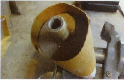
Photograph 7 – Fused end disk in the paper can.
