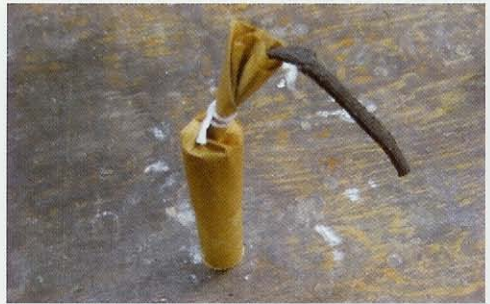
Photograph 5 – The nosed whistle-time fuse.
