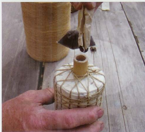
Photograph 32 – Inserting the bared section of the leader into the whistle.
