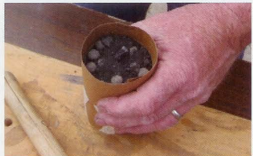
Photograph 17 – Stars and polverone up to the cardboard liner.
