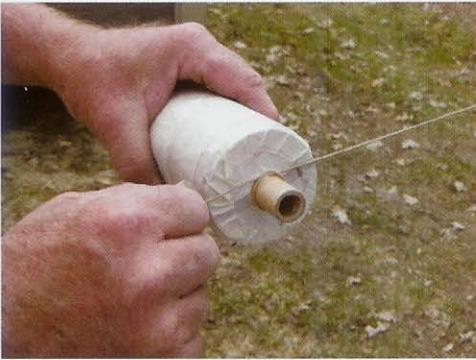
Photograph 23 – Tying the string to the whistle-fuse for spiking.
