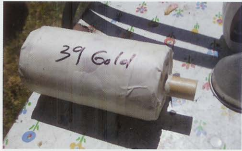
Photograph 22 – The shell wrapped with masking tape.
