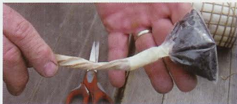
Photograph 30 – The lift charge and leader ready to be attached to the shell.
