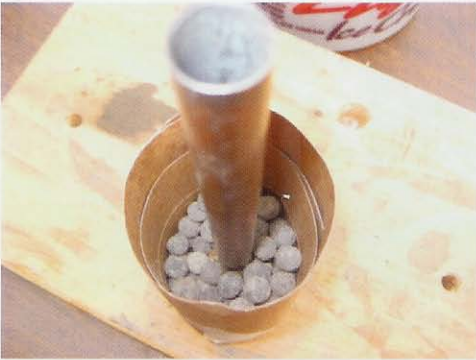
Photograph 13 – Adding stars around the canulle.
