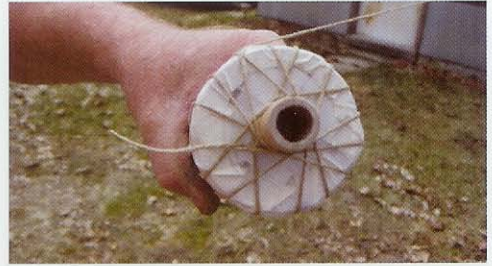
Photograph 25 – A top view of the shell with vertical spiking completed
