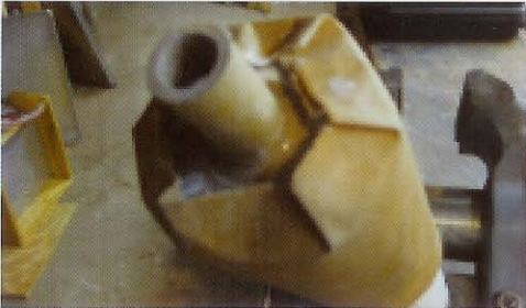
Photograph 8 – Pleating the overhanging paper over the end disk.
