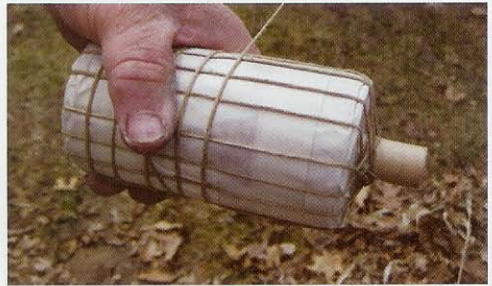
Photograph 27 – Winding on the horizontal spiking to form squares.
