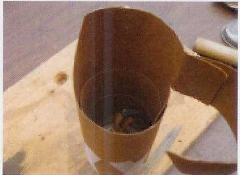
Photograph 12 – Trimming the case to one-inch above the liner.
