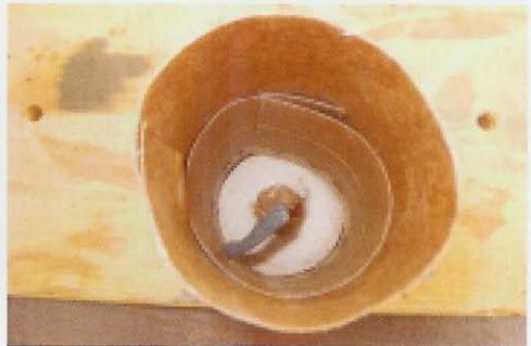
Photograph 11 – Thin cardboard liner inside the shell casing.
